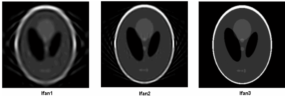
Reconstructions of the Head Phantom Image from Fan-Beam Projections
